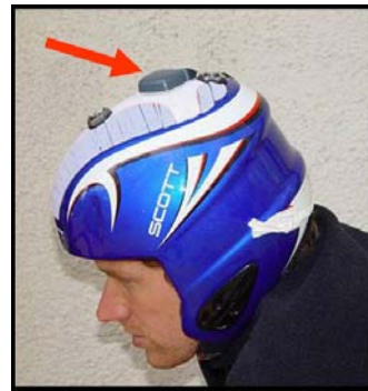
Figure 4. Small antenna (here fixed on the helmet); dimensions: 9 x 9 cm; weight: 90 g
