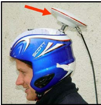
Figure 3. Original antenna; dimensions: diameter 21 cm; weight: 300 g
