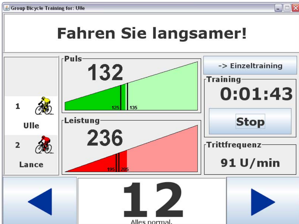
Figure 6: For each cyclist, heart rate (“Puls”), power (“Leistung”), cadence (“Trittfrequenz”) and time as well as the position are monitored on the touch screen of the UMPC. On top, feedback as well as advice from the TCTS is displayed (e.g. “Drive slowly”/“Fahren Sie langsamer”). The bottom line shows the current rate of perceived exhaustion on the Borg scale. With the two buttons on the left and the right, cyclists can adjust their rating.
