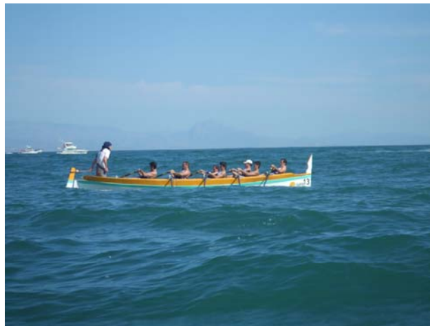
Figure 1. Characteristics of “Falucho o Mediterranean Llaüt”: Total length 812 m; mast bow 99m; mast stern 83m; midship section mast, 81m; midship section tug .237m and midship water line tug. 173m. 8 rowers plus a coxswain, having five fixed seats to double rowers except the coxswain.
