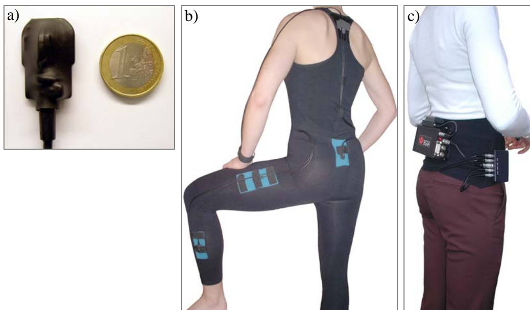
Figure 2. Sensor size (a), sensor attachment (b) and visible hardware components (data logger and sensor box) of the system worn under the clothes (c).
