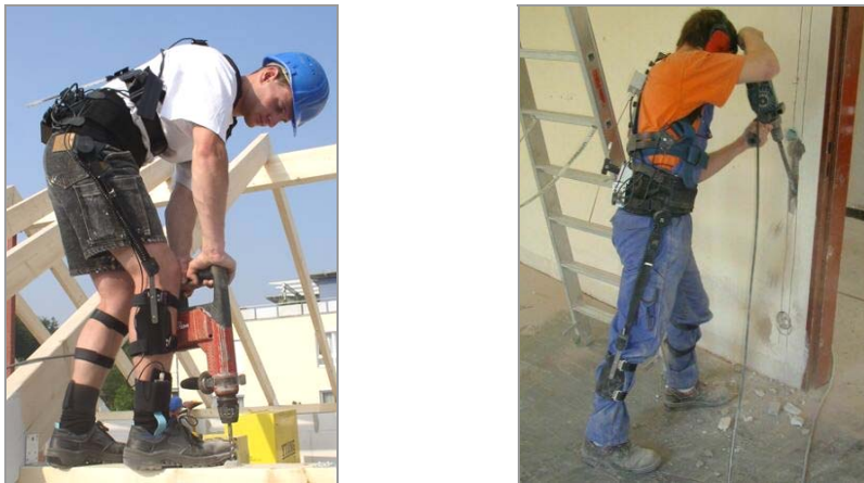
Figure 1. Application of the CUELA measuring system on a carpenter's and an electrician's workplace.
