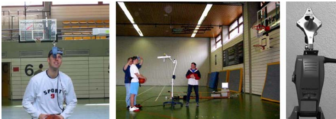
Figure 4. Use of the head mounted display in the sports hall. The line of sight is detected by a localization system. The tracker is attached to the head mounted display.
