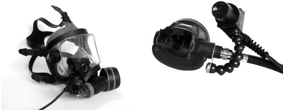
Figure 1: The HUD fitted to a full-face mask and to a second stage regulator
