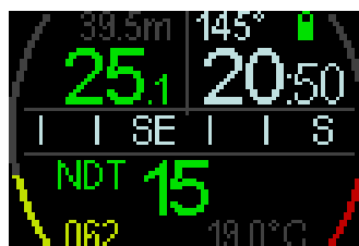
Figure 2: Typical display as seen by the diver. In this case maximum depth 39.5m, current depth 25.1m, dive time 20:50min, heading SE 145°, battery OK (green), remaining no decompression time 15min, cylinder pressure 62bar, ascent rate warning (red >10 m/min) and temperature 19°C.
